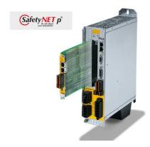
Caption: The new safety card PMCprotego S3 from Pilz expands the drive-integrated safe motion solution, adding further safe motion monitoring functions in accordance with EN 61800-5-2. With these functions it is now possible to configure an application-specific error reaction in advance, flexibly and individually via the engineering tool PASmotion. That reduces machine downtimes. (Photo: © Pilz GmbH & Co.KG)
