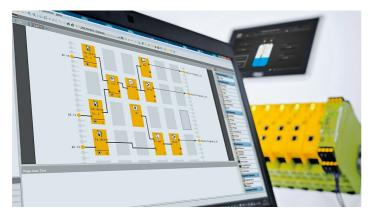
Caption: For the configurable safe small control system PNOZmulti from Pilz, a new application simulation is available from Version 10.9. Users can test the configured user program even before commissioning, and thereby save time and costs during configuration.
