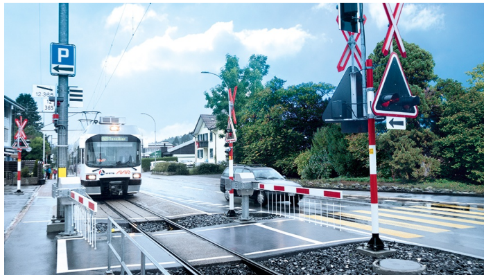
Caption: The PSS 4000-R automation system is used throughout Europe to secure railways crossings (with or without barrier protection), for example, and assumes control and safety tasks.
