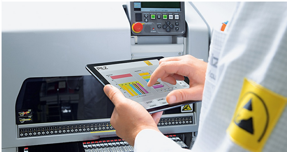
Caption: Small controllers PNOZmulti can now be linked directly to the visualisation software PASvisu. As a result, the full function range of the software is available, including the diagnostic option.
