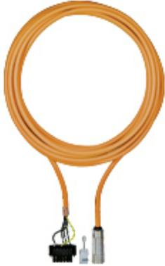
Cable for PMCprotego and motor with connector design assembled on both sides with connector <> round connector 8-pin No. of wires and cross section (4 x 4.0 + (2 x 1,5)) Trailing, length: 20 m.
