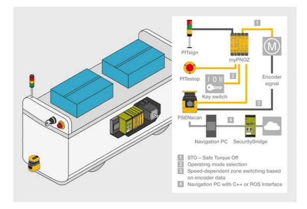
Example of protective measures on an AGV
