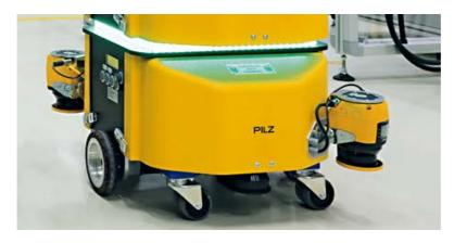
In this example, the AGV is moving in an aisle at one side of a production hall to deliver material needed for a machine. The aisle is wide enough to be assessed as a normal "operating zone" with the AGV operating at full operation speed, since clearances of 500 mm or more to each side are achievable.
