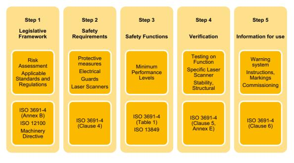
Figure 1: Process for an individual AGV incl. examples of references
