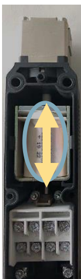
Figure 9: Interior view of electromechanical guard locking device PSEN me5
