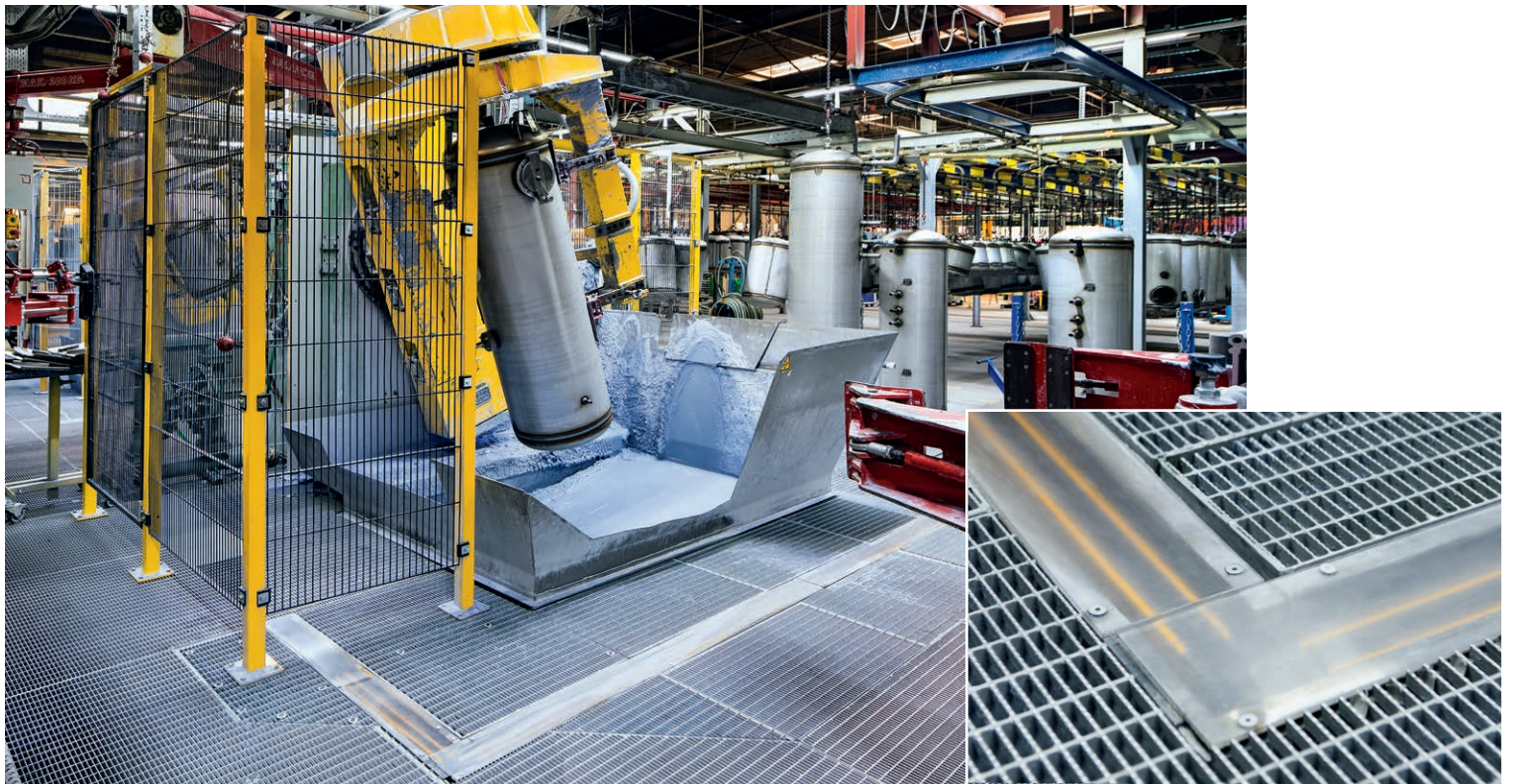
The area around the individual positioner is accessible from three sides. Easily identifiable: a tank is being fed in the background. After successful machining, a gripper (red) picks up the tank. The transmitters on PSENOpt II light curtains from Pilz have been embedded into the floor for barrier-free, safe access to the plant.
