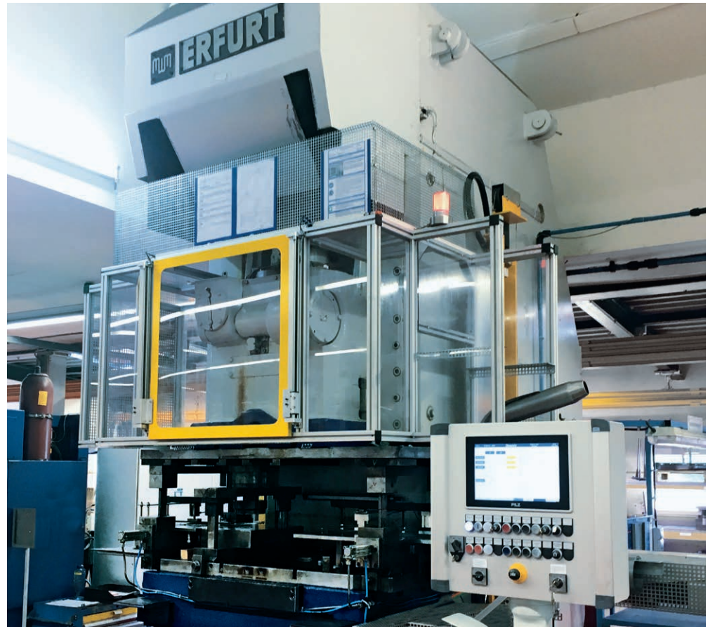
After the retrofit: The panel version of the Pilz motion control range PMI 6 primo offers professional control, visualisation and diagnostics in one system.
