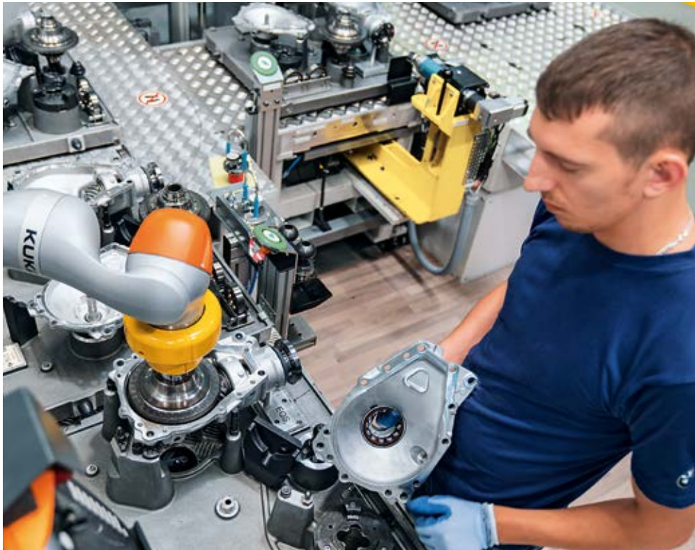
Human-robot collaboration in axle drive assembly, BMW Group Dingolfing plant: BMW Group is working together with Pilz on safety.
