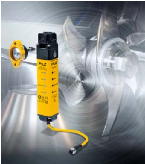
The safety gate system PSENmlock from Pilz combines two functions: safe guard locking and safe interlocking in a single device – especially for machinery with dangerous overrun (such as rotating spindles, blades).
