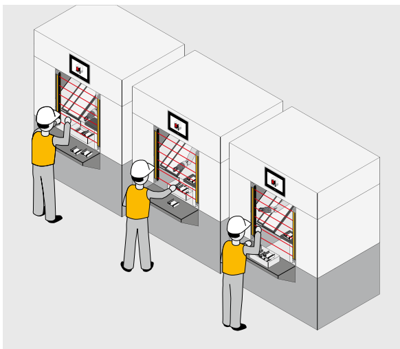
Light curtain PSENopt II with integrated coding for a flexible arrangement with close proximity.
