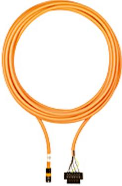
Power cable; Cable assembled on both sides Connector <> con.15 round connector 9-pin SpringTec; No. of wires and cross section (4x1,0+1x(2x1,0))suitable for PMCprotego D.01-24 and the motors PM Ctendo SZ.3x; Length 5m.
