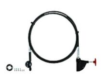
Push/pull cable release for the safety gate system PSENmlock, cable length 0.5m, package content = Push/pull cable and operator element. Ensure that this version is installed as straight as possible. With the escape releases with order no. 570466 and 570467 bending the push-pull cable can reduce the functionality and the service life.
