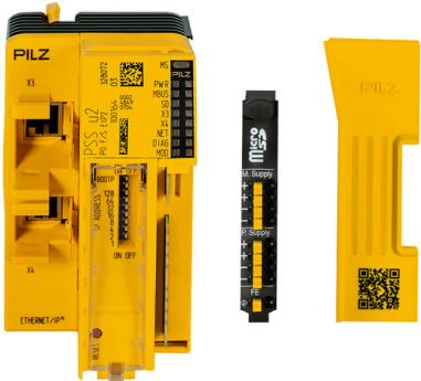
PSS u2, head module, performance index P0, control system I/O, failsafe and standard, 2 RJ45 ports, EtherNet/IP adapter with CIP Safety, supports BOOTP, integral power supply, infeed module supply 24 V DC 1.2 A, infeed periphery supply 24 V DC 8 A, potential isolation, connection functional earth, for microSD card integrated in the terminal block, with protective plate.
