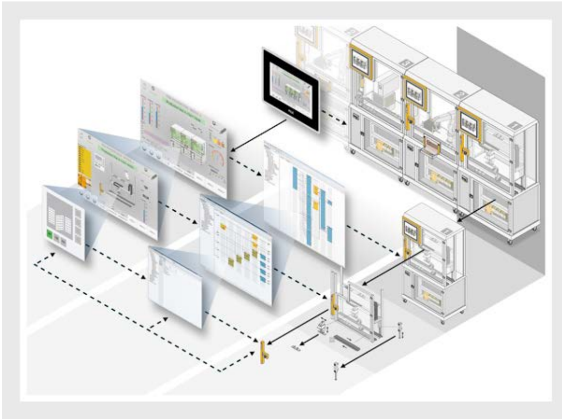
Plants can be broken down into manageable, independently functioning units.
