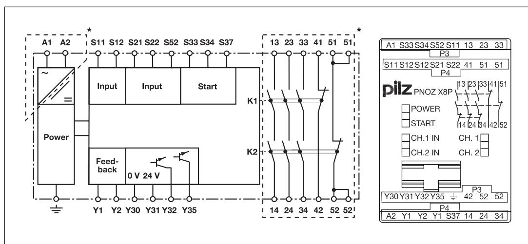
\*Insulation between the non-marked area and the relay contacts: Basic insulation (overvoltage category III), Protective separation (overvoltage category II)
