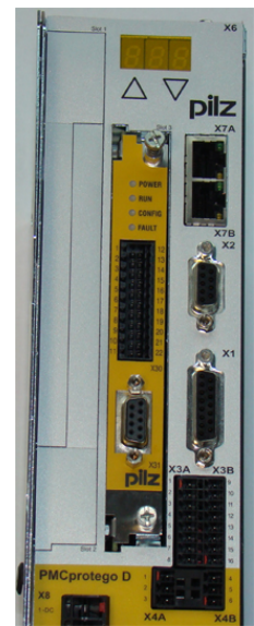
5. Plug in the safety card and tighten the screws
