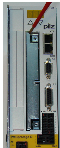
3. Break the top link and lever out the cover plate
