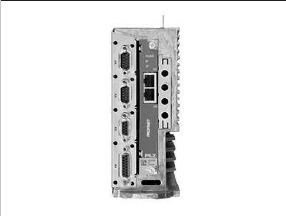
Fig.: PROFINET expansion card installed in PMctendo DD5
