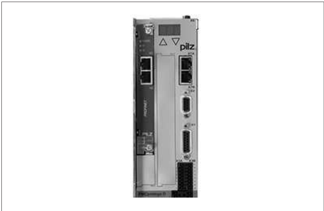
Fig.: PROFINET expansion card installed in PMCprotego D
