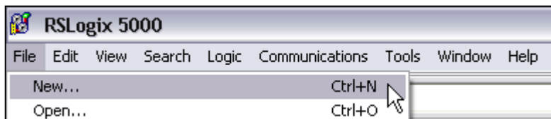
Fig. 6: RSLogix 5000 – Create new project (1)
