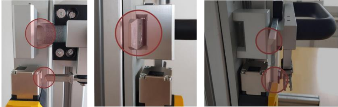
Figure 11: Fault exclusion due to leading bolt
