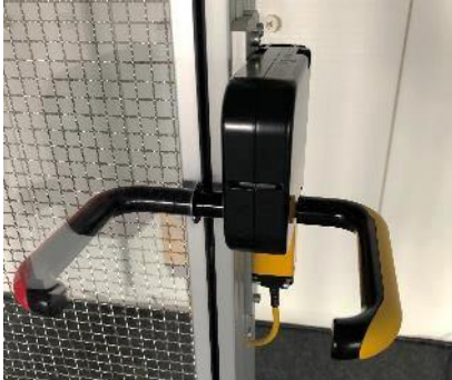
Figure 24: Escape release integrated in the handle, PSENmlock door handle module (red handle) as example
