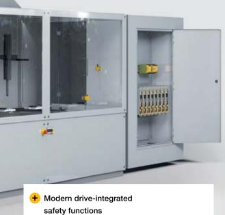
for increased productivity and reduced maintenance work, up to the highest safety level PL e and SIL 3
